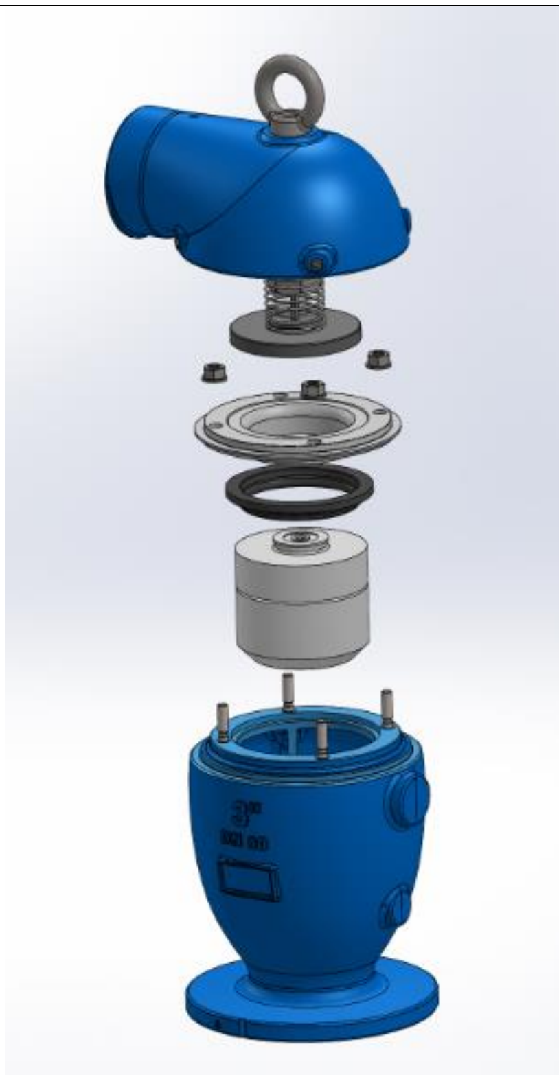
Picture #5 – assembling the specialized top plate and placing the Inflow Prevention kit above the top plate.
