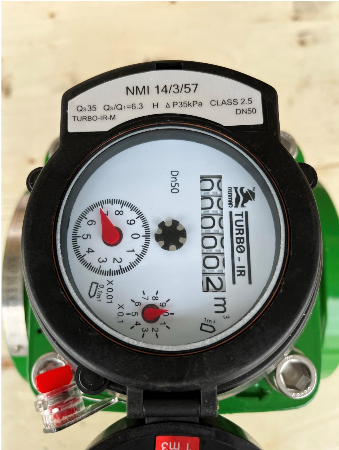
Example of required markings
