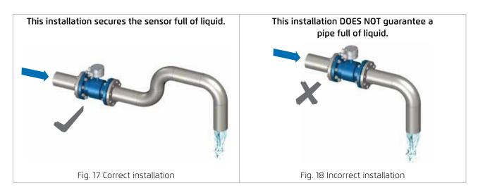
We recommend installing the sensor on a vertical/sloped pipe with an upward flow direction (Fig. 19) to minimize the wear and deposits in the sensor. Avoid the installation on vertical pipes with free exit (Fig. 20).
