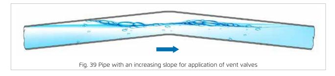
A minimum slope in an ascending flow of 1: 500 or higher is recommended in order to stimulate the entrapped air pocket to move away from the meter.
