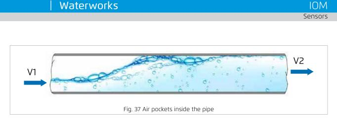
The greater the diameter of the pipe, the higher the speed of the liquid will be required to move the air pockets away from the flowmeter.
