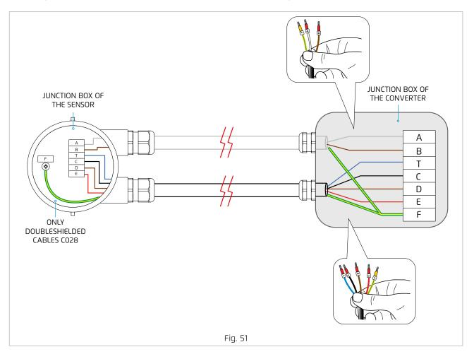
Info: If cables in the coil are used, always use the ferrules for the connections in the terminal board and adequately insulate the shields.
