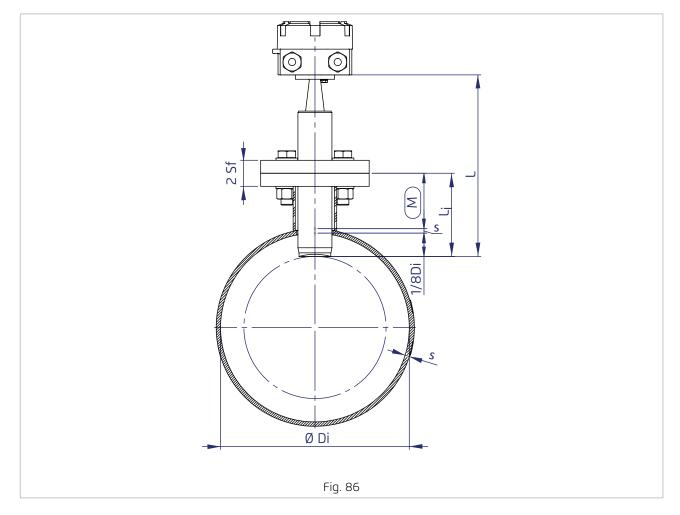
The insertion depth I can be determinated using the following formula:
