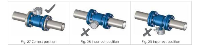
(\*) Note: Insertion meters can also be installed horizontally.
