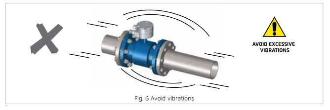
Install a suitable anti-vibration protection if vibrations occur.
