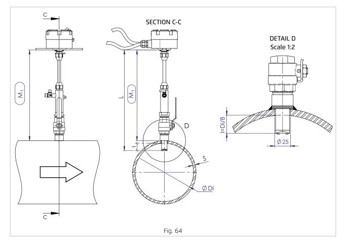
The insertion depth I can be determinated using the following formula:
