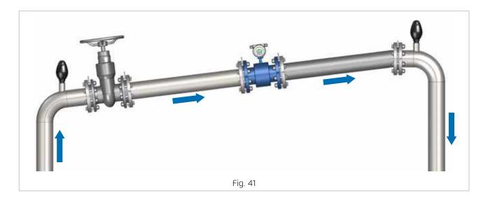
The design of the vent valve is essential to ensure that the entrapped air pockets are released.
