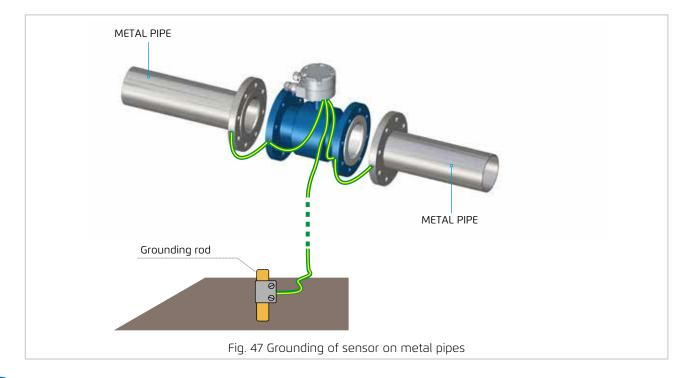
In the case of metal pipes with an insulating coating, follow the instructions for plastic pipes.
