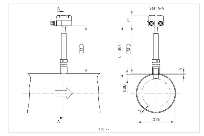
The insertion depth I can be determinated using the following formula:
