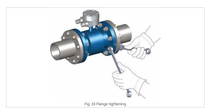
Carefully follow the instructions given in the diagrams. Check the correct centering of the sensor before you tighten the flanges and proceed following the steps described here.
