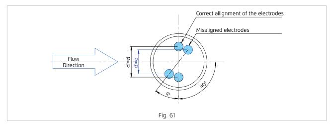
It is essential to carefully position the electrodes in relation to the direction of the pipe.
