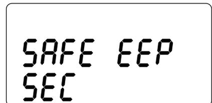
The firmware or the EEPROM data checksum (parameters and/or totalizers) has failed the last integrity check; no further measurement will be performed.
