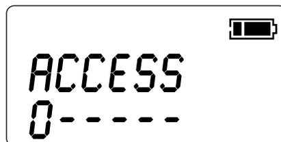
to increase / decrease the current digit value use P4 / P3; move to the next digit with P2. When the last digit is entered, a further presson of P2 will unlock the access to the function selection if the entered password is correct, otherwise the digit will scroll back to the first one
