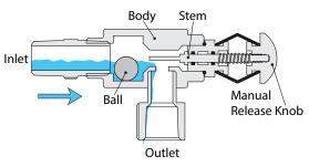
**Open:** The Automatic Drip Check drains accumulated water/fluid from condensation/system leakage from the piping.
