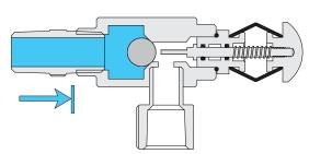
**Closed:** When the system piping suddenly fills with water/fluid the drip check closes.
