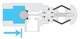
**Closed:** When the system piping suddenly fills with water/fluid the Automatic Drip Check closes.
