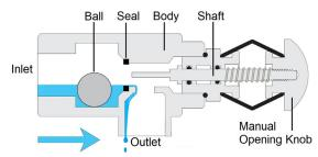
**Open:** The normally open Automatic Drip Check drains accumulated water/fluid from condensation/system leakage from the piping.
