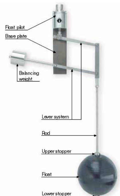
Figure 2: 67 Float Pilot Valve
