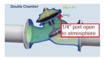
To minimize the minimum head loss in the valve the inner spring is removed. Typically, the V port plug is used for regulation should the range of flows required is from zero upwards. If using the PRV for medium to higher flows only, the valve can be configured with a flat disc that increased the flow capacity slightly.
