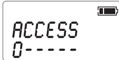
to increase / decrease the current digit value use P4 / P3; move to the next digit with P2. When the last digit is entered, a further pression of P2 will unlock the access to the function selection if the entered password is correct, otherwise the digit will scroll back to the first one
