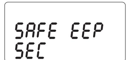
The firmware or the EEPROM data checksum (parameters and/or totalizers) has failed the last intergrity check; no further measurement will be performed.
