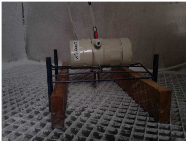
Verifica del grado IP 6X / IP 6X degree test
