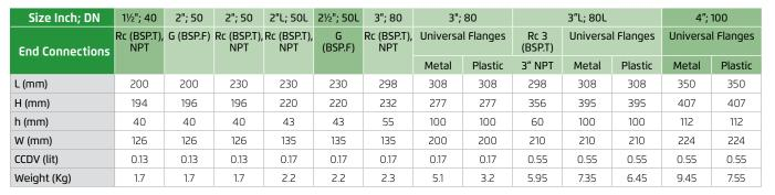
CCDV = Control Chamber Displacement Volume • BSP.T = Internal Threaded • BSP.F = External Threaded
