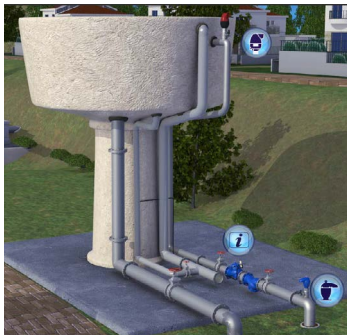
Picture 4.5 - Elevated reservoir
