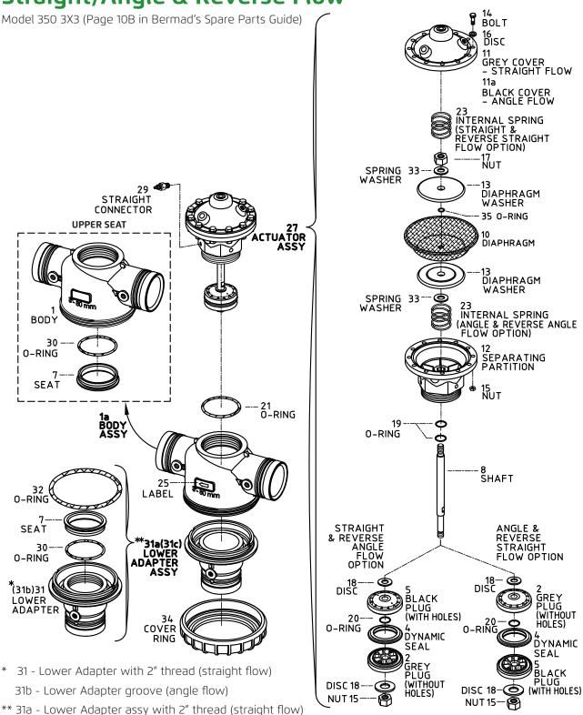
31c - Lower Adapter assy groove (angle flow)
