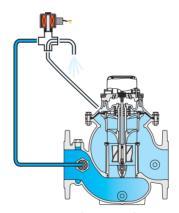
Solenoid Closed Hydrometer Open
