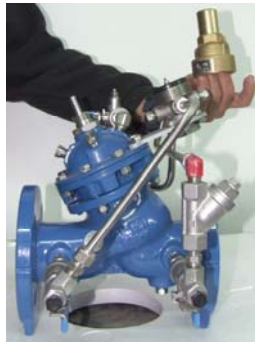
3.2. Replacing Pilot Cover
