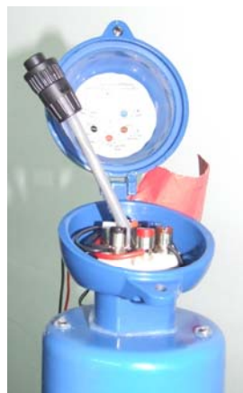
3.12. Connections cover opened - wires pulled
