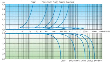
The air flow charts were created in Kg/s from laboratory tests and numerical analysis, then converted using a safety factor.
