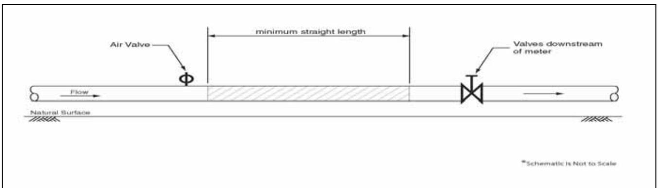
\*\* Meter is to be installed within the "minimum straight length" section of pipe. In the absence of other recommendations by the meter manufacturer, the length of upstream pipe section must be at least ten times the pipe diameter and the downstream pipe section must be at least five times the pipe diameter.
