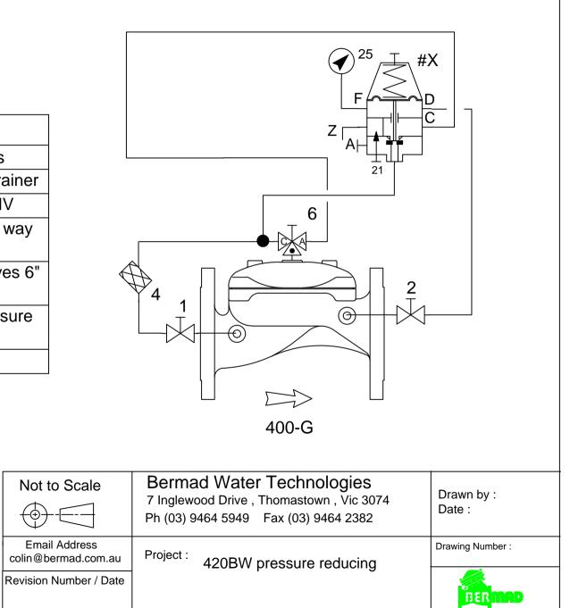
Suitable build for 400 series valves from 6" up to 12" for irrigation applications
